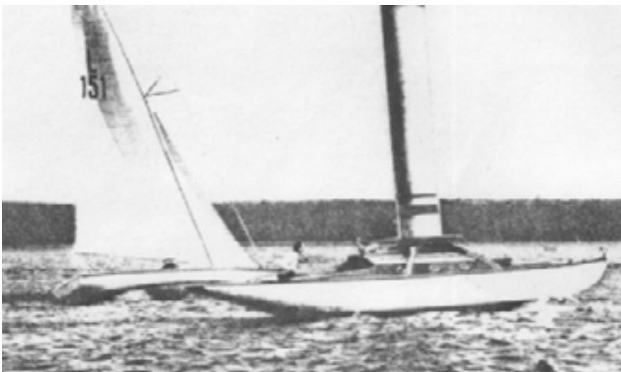
FIGURE 3: Kiernan and Hastings rotor yacht
