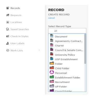
3. Select a Record Type from the displayed list of Record Types. If the Record Type is not listed, type in the name of the Record Type and then select it from the displayed list. To move through the list of Record Types, you can press the **DOWN** or **UP** arrow keys on the keyboard and press **Enter** to confirm the selection.
