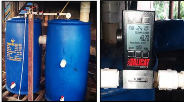
The biogas digester that was constructed (left) and the flow meter used for measuring the amount of biogas produced per day (right).
